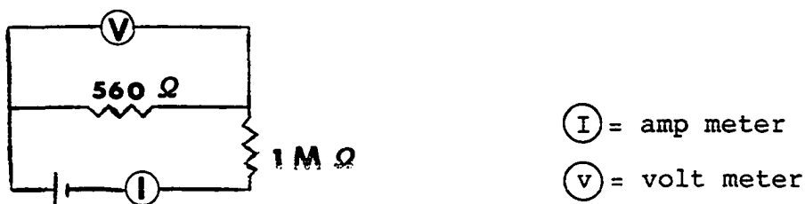
Figure B-1. Circuit diagram for cryostat temperature determination
